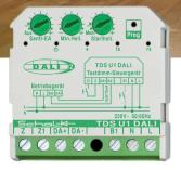
The minimum brightness, start brightness and on/off ramp can be adjusted. In addition, the power-on behaviour can be specified. The DALI-2-certified TDS U1 DALI control unit can supply up to 35 DALI control gear units via the integrated power supply.
