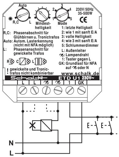
Terminals L and  $\textcircled{x}$  are duplicated. In thermally problematic installations, heat dissipation can be improved by additional connection of these terminals. If terminal GK is wired to N, the pushbutton line can drive up to 15 mA glow-lamp current.
