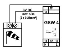
Fig. 1: Wind sensor connection
