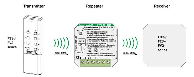
All radio transmitters of the device series Fx3 (= FS3, FD3) and FV2 are compatible with the radio repeater FV2 R
