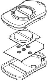
Insert key mat (note the grooves on the housing edge!)
