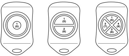
Important: only with the FS3 HS 4 can all 8 keys of a large handheld transmitter be simulated (FS3 HS 2: only key 1 or 5, FS3HS 2: only key 1+2 or 5+6)
